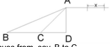
As the rope is pulled a distance x, the boat moves from, say, B to C. So CA = BA - x
